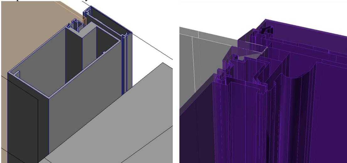
245 **Figure 2. Window frame details: (a) Revit MEP, (b) Rhinoceros 3D.**
